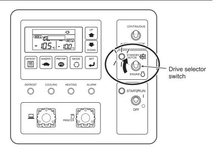
1 Connect the socket of the refrigeration unit to the commercial power supply.
